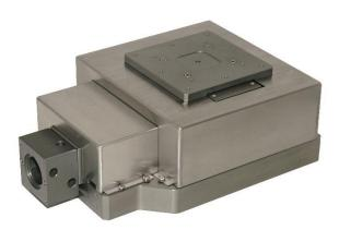
Elevator Stage ES-200 is designed for vertical Z-axis applications requiring extremely fine incremental up-down motions. The ES-200 offers high resolution, high repeatability and high mechanical stability. The dual column guide and the patented single plane wedge drive achieve exceptional narrow bandwidth trajectory.
